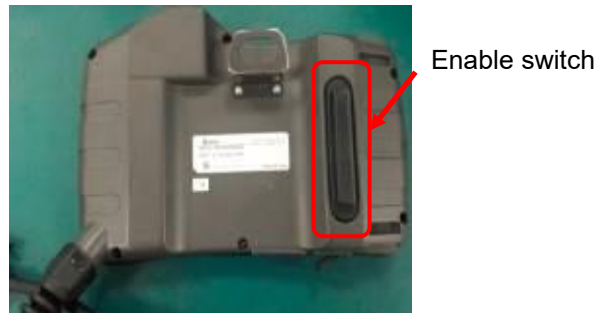
Figure8. 37 Location of the enable switch behind the teach pendant
