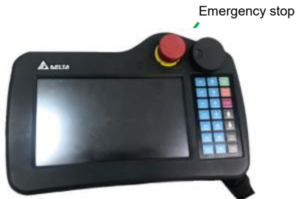
Figure8. 36 Location of the emergency stop button on the teach pendant
