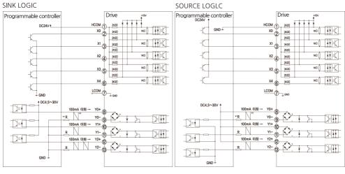
\* 1) Limited resistance In the case of 24V DC:  $680\Omega \sim 2.7\Omega$  (2W) In the case of 5V DC:  $150\Omega \sim 560\Omega$  (0.5W)
